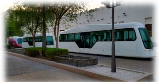
City Cars (3) autonomously coupled, 300 passengers
