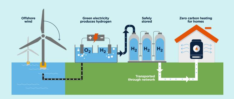
H100 Fife will be the world's first 100% green hydrogen-to-homes network for heating if proposals are approved by the energy industry regulator Ofgem. An initial 300 homes in Levenmouth, Fife, will have access to hydrogen for heating and cooking within two. The project will start construction in late 2020/early 2021 and is intended to provide critical evidence for a zero carbon energy source, helping to inform the UK's long-term policy decisions for decarbonisation of heat.
